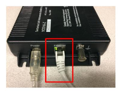
14. If connecting directly to the PC, connect the gray Ethernet cable to the StarTech Ethernet to the USB adapter.
