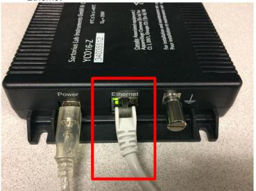
7. Connect the other end of the gray ethernet cable to the StarTech ethernet to USB adapter
